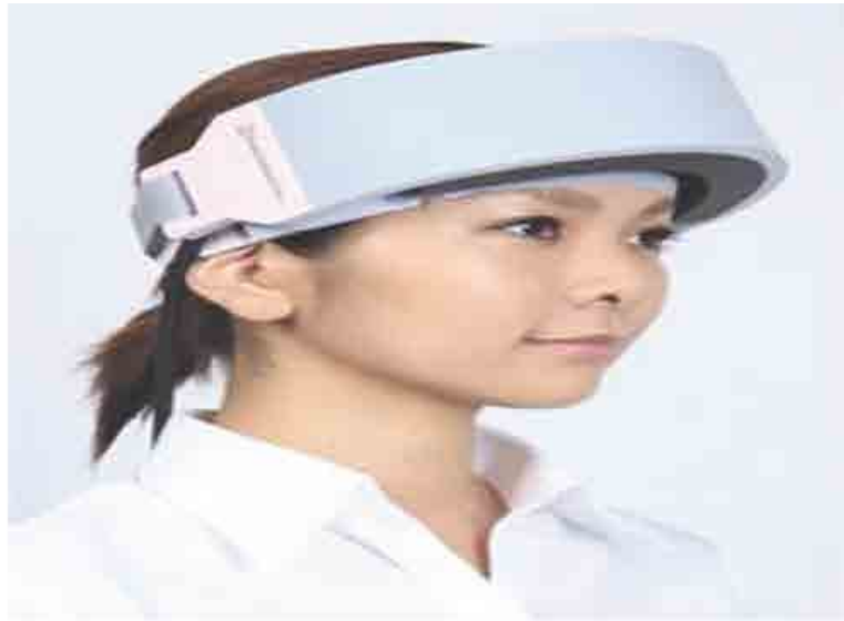
Figure 1 -flow of the blood at the frontal part of the brain was measured using 16-channel optical encephalography using the OEG-APD series instrument developed for encephalography
