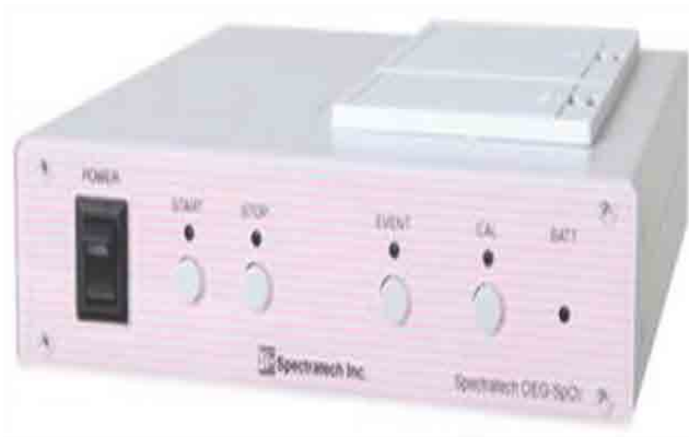
Figure 2: 16-channel optical encephalography using the OEG-APD series instrument developed for encephalography
